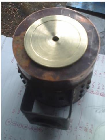
The smokebox door is a simple brass  $\frac{1}{4}$  inch (6mm) plate at  $3\frac{1}{2}$  inches (87mm) in diameter with a  $\frac{1}{16}$  inch (1.5mm) lip cut away at 3 inches (75mm) in diameter at the rear to locate it against the smoke box front plate and the front face rounded off for appearances sake.
