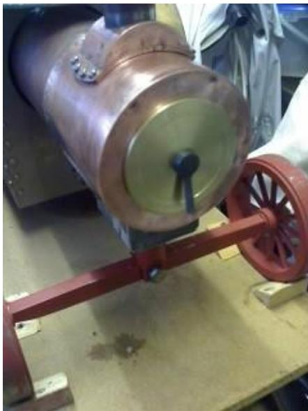
In this live-steam model we need only two of those functions as it serves only to support the chimney and have the steering mounted under it, plus it also provides the necessary appearance of a conventional live steam traction engine.
