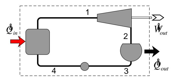
As a heat engine:-  $Q_{in} = W_{out} + Q_{out}$
