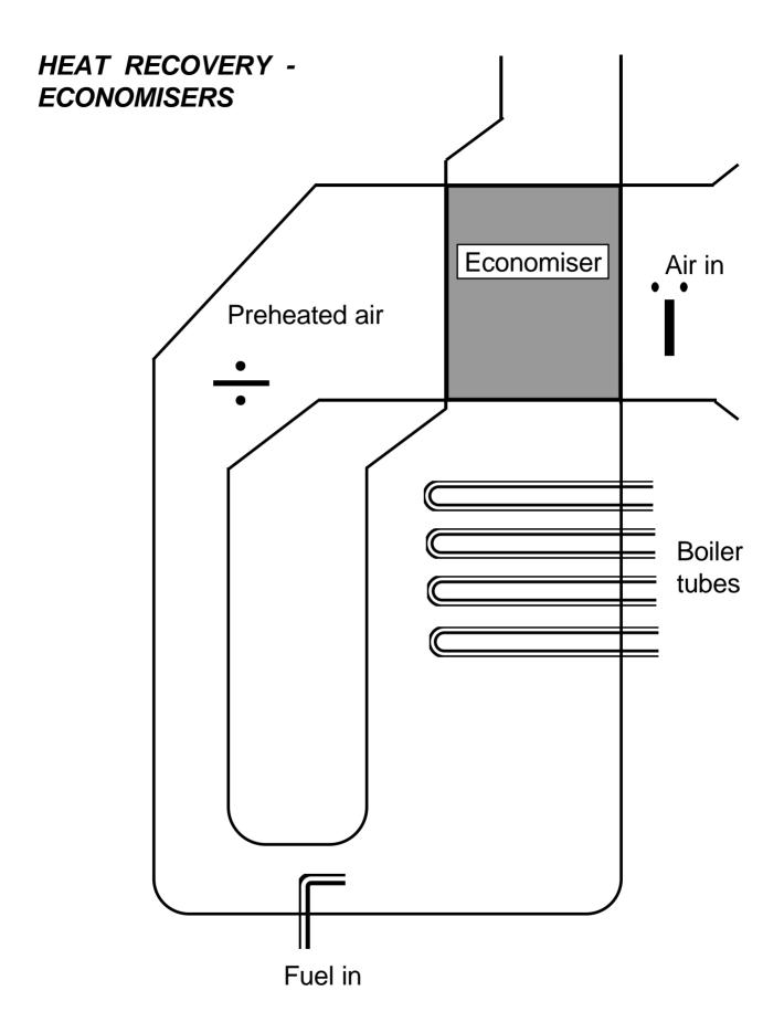
An economiser (air-to-air) preheats in-coming air using 'waste' heat in the flue gases
