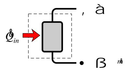
We may analyse the boiler as a steady state open system using the SSFEE:
