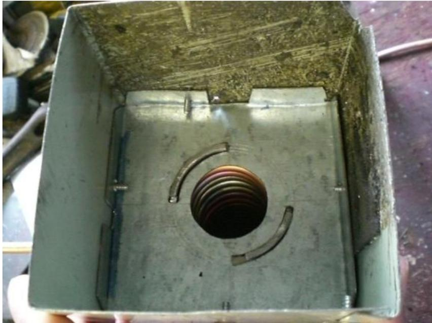
Also at the bottom two grooves need filing away to allow two tongues at the base of the boiler tube to stick through the bottom plate as can be seen in this picture, that way keeping the bottom of the boiler barrel central once again. Fine, it is not sitting level here, but it is central as required.
