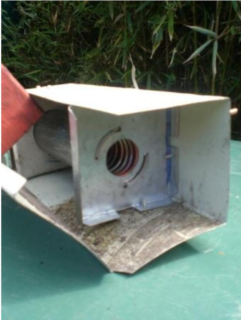
This second tube, let's call it the boiler barrel, was 20cm long with an outside diameter of 50mm - the wall thickness was 3mm if I remember rightly - it was a lump of tube I had to hand, but as this part does not need strength using half that thickness is fine.
