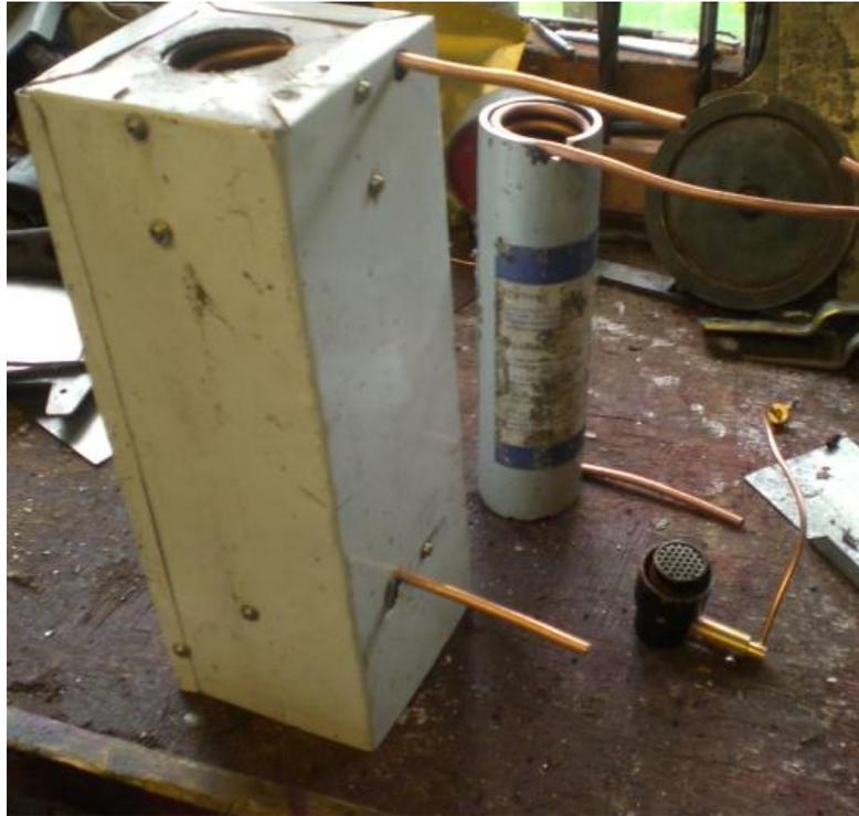
Here you can see the layout of the piping sticking from the boiler shell with a similar boiler tube containing a fire tube (although wound the opposite way to produce a matched pair initially) to the rear. These boiler tubes were originally pressure vessels for carbon dioxide for beer and wine making purposes with both the top and bottom removed.
