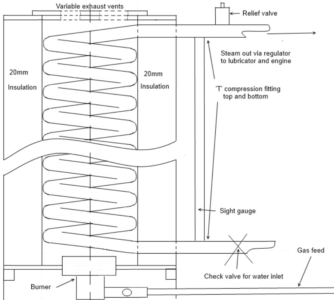
My first boiler was built from gathered together bits and pieces, using nothing more than a hammer, screwdriver, hacksaw and files, along with a drill and various bits. It was very inexpensive to produce, the costliest parts being the heating arrangement, with the copper tube and fittings adding to the price. The remainder were recovered from an old computer and an old microwave which were both destined for the tip. These were used for the bodywork.
